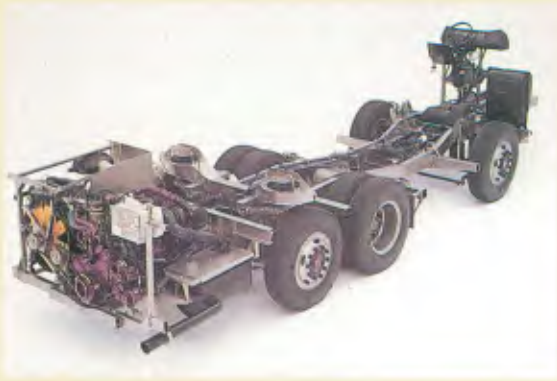
Chassi-modelo/ Chasi-modelo /Chassi model: B12 6X2 Motor-potência/ Motor-potencia /Engine power: TD 122 FL/396 cv. Entre-eixos/ Distancia entre los ejes / Wheelbase:3,0 m (Buggy)
