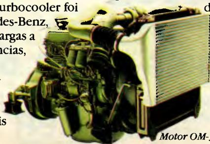
Motor OM-366 LA, com turbocooler.
