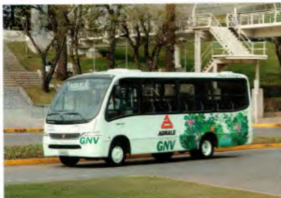
Micro Agrale, com motor a gás Cummins 6BG-5.9 Plus
