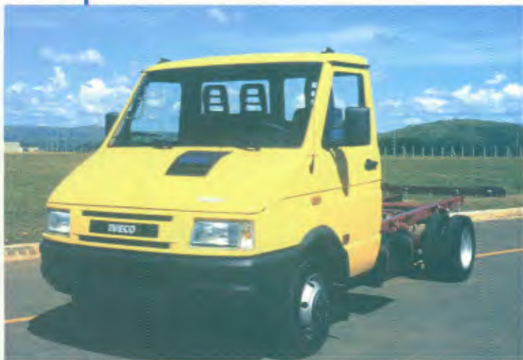
Modelo: Daily chassi-cabine Entre-eixos: 3.200 mm, 3.600 mm, 3.950 mm Motor: Iveco 8140.23, 103 cv a 3.600 rpm, e 8140.43, 122 cv a 3.600 rpm PBT: 4.000 kg, 5.200 kg
