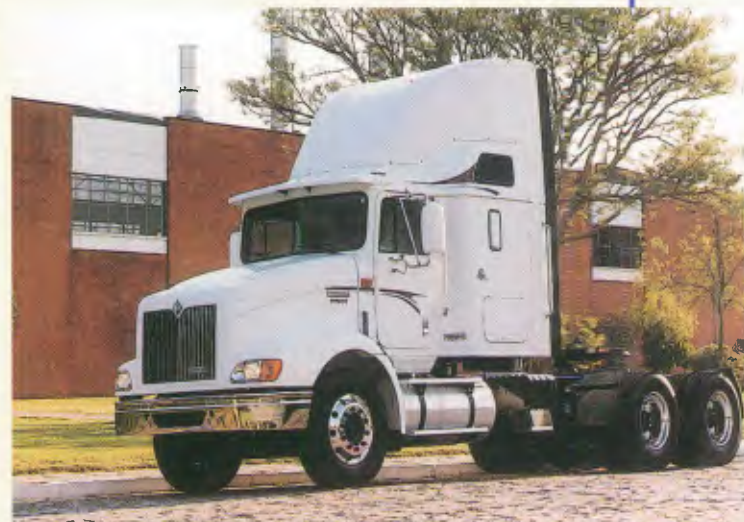
Modelo: 9200 Entre-eixos: 4.490 mm Motor: Cummins ISM 380E, 380 cv a 1.900 rpm, Cummins ISM 405E, 400 cv a 1.900 rpm PBT: 23.000 kg
