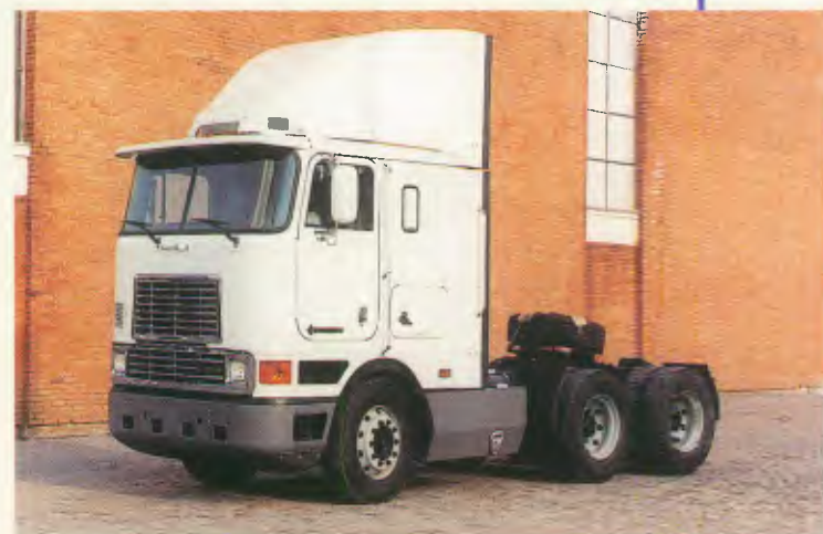
Modelo: 9200 Entre-eixos: 4.490 mm Motor: Cummins ISM 380E, 380 cv a 1.900 rpm, Cummins ISM 405E, 400 cv a 1.900 rpm PBT: 23.000 kg
