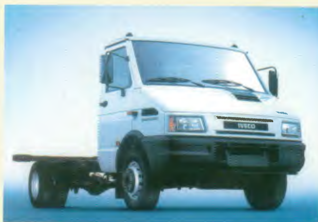
Modelo: Daily RD chassis 60.12 Entre-eixos: 3.300 mm, 3.600 mm, 4.180 mm Motor: 122 cv a 3.600 rpm PBT: 3.950 kg, 4.010 kg, 4.040 kg
