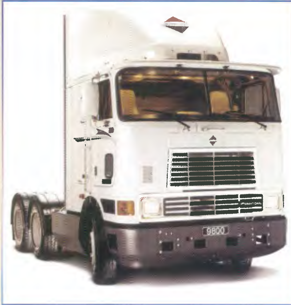
Modelo: 9600 6x4 Entre-eixos: 3.150mm+1.400 mm Motor: Cummins ISM 405E, 404 cv a 1.900 rpm PBTC: 60.000 kg
