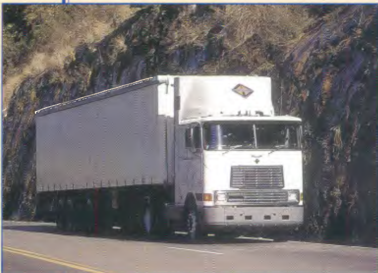
Modelo: 9800 4x2 Entre-eixos: 3.760 mm Motor: Cummins ISM 380E, 379 cv a 1900 rpm PBTC: 45.600 kg
