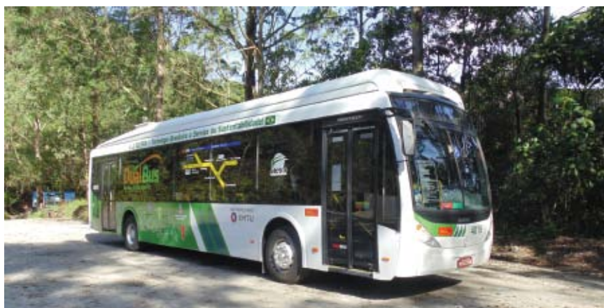
In Eletra Dual Bus, the traction system can be powered by multiple power sources
