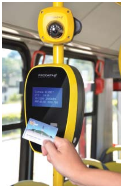
Prodata: smart validator installed on Porto Alegre buses
